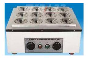
Standard double wall construction, inner being of stainless steel outer of m.s. duly staving paint finish and gap filled for temp. insulation with glass wool. The cover with 75mm (3") holes with concentric rings. Temp. range 5<sup>o</sup>C above ambient to 95<sup>o</sup>C controlled by a thermostat. Heating is attained by an immersion type element with accuracy of  $\pm 1^{\circ}$ C.
