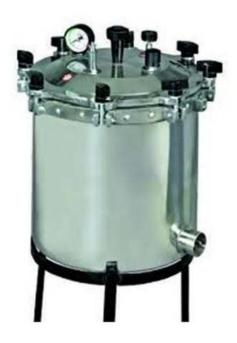
Suitable for general laboratory use sterilization. Stainless steel or aluminium vertical body having no joints. Pressure range 15psi to 18psi. Domed cover can be sealed by a jointless gasket which is clamped to the vessel by wing nuts by hinged bolts which engage. Spring loaded safety valve has threaded cap for pressure adjustments. Supplied complete with plug and cord and suitable to work on 220V AC 50 Hz single phase.
