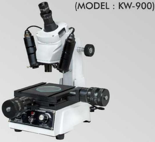
This Microscope has X-Y movement on ball bearing slides, having micrometer (50mm dia) Least Count - 0.01 or 0.005mm with goniometer. Fixed magnification 30x. 150x150mm stage, and 360° rotary head. Having both transmitted & incident light. This comes packed in a wooden box.
