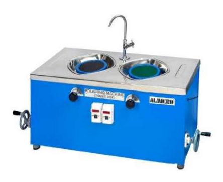
This is a simple and convenient machine for rough and fine polishing of metallurgical specimen. This specimen after mounting and after being polished by hand on emery paper is polished on this machine.
